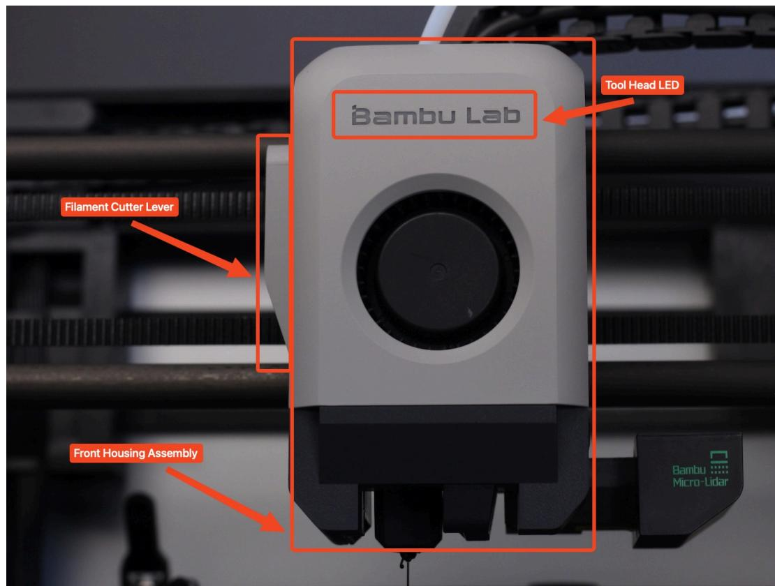
The extruder is responsible for pulling the filament from the spool and feeding it to the hotend, where it is melted and pushed through a small nozzle to generate the printed model. It's also one of the most important components of a 3D printer, as it needs to accurately control the amount of filament pushed through the hotend.
